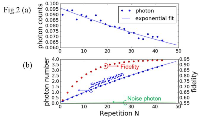
Fig.1 Quantum circuit for the conventional (upper) and single-shot (lower) measurements. Fig.2 (a) Averaged photon counts of Nth measurement decaying by the relaxation of the nitrogen nuclear spin. (b) Accumulated counts of the signal and noise photons and the corresponding measurement fidelity.
