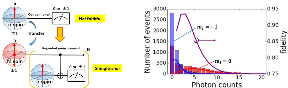
Fig.1 Quantum circuit for the conventional (upper) and the deterministic (lower) measurements. Fig.2 The distribution of the photon counts and the corresponding fidelity to distinguish the nuclear spin state.
