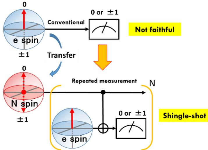
Fig.1. Quantum circuit for the conventional (upper) and single-shot (lower) measurements.
