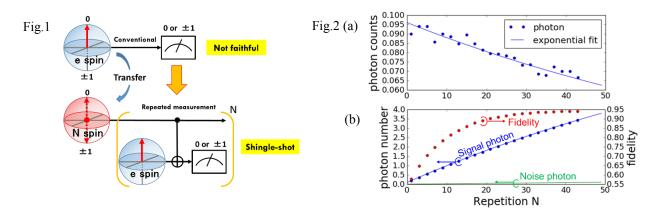
Fig.1 Quantum circuit for the conventional (upper) and single-shot (lower) measurements. Fig.2 (a) Averaged photon counts of Nth measurement decaying by the relaxation of the nitrogen nuclear spin. (b) Accumulated counts of the signal and noise photons and the corresponding measurement fidelity.
